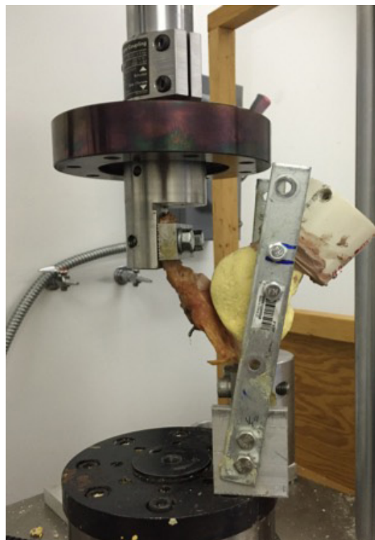
Figure 3. Representative experimental setup. Repaired specimen is attached by clamps inferiorly to the MTS Bionix 858 (MTS Systems) load cell and superiorly to the MTS hydraulic piston. A distal femur sawbone was bracketed to the load cell and secured to provide a 45° hinge point on the posterior surface of the patella.
