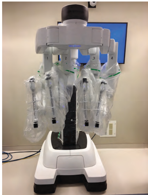
da Vinci Xi Surgical System (Intuitive Surgical, Sunnyvale, California); patient side cart.
