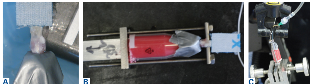
Figure 3. (A) Supraspinatus tendon under a 0.2-N tare with a 3-mm gauge block. (B) Humeral shaft embedded in polymethylmethacrylate with the head protruding outward and secured by the plate. (C) In biomechanical testing setup, the tube is angled 15° from vertical, which simulates 105° of shoulder abduction. The shoulder is continuously bathed with a 0.15-M saline.
