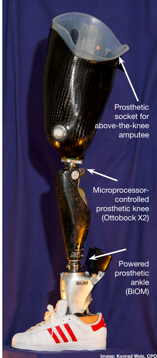
Figure 1. The BiOM T2 Foot and Ankle Prosthesis, Providing Dorsi- and Plantarflexion.
