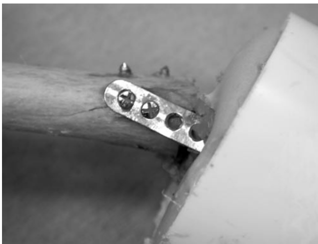
Figure 7. Wrist internal fixation system (TriMed, Valencia, Calif) loaded to failure. Note widening of osteotomy site volarly and dorsal translation of distal fragment.
