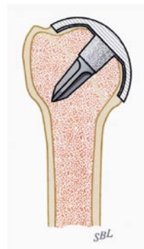
Figure 2. In the same resurfacing implant shown in Figure 1, the proximal humerus is reamed to fit the back of the implant, which has a flat, porous-coated surface for bone ingrowth. Illustrator, Steven B. Lippitt, MD.
