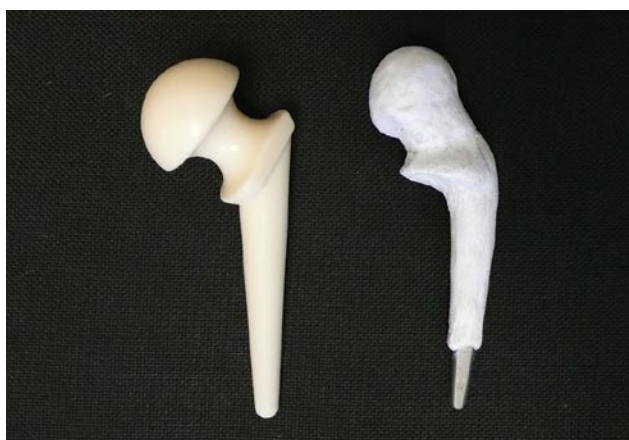
Figure 2. Commercially available spacer (on left) and handmade construct with prosthesis skeleton (on right; tip broke during testing), showing difference in surface finish.
