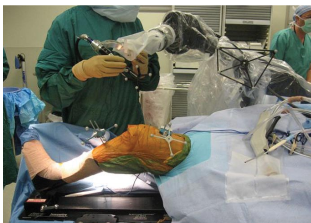
Figure 2. Robot registration is performed after conventional positioning and sterile draping.
