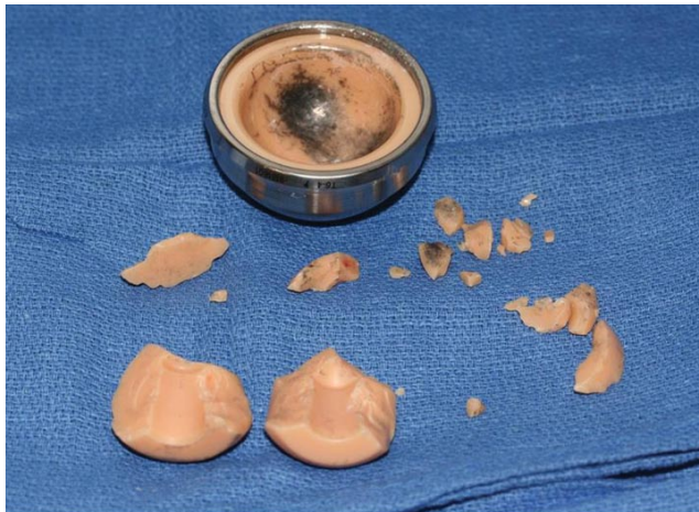
Figure. Metal-backed ceramic acetabular component and fractured ceramic femoral head.
