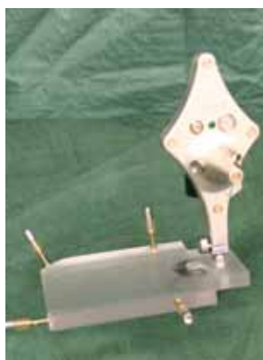
Figure 1. Multimodality registration object (length, 8 cm; width, 8 cm).
