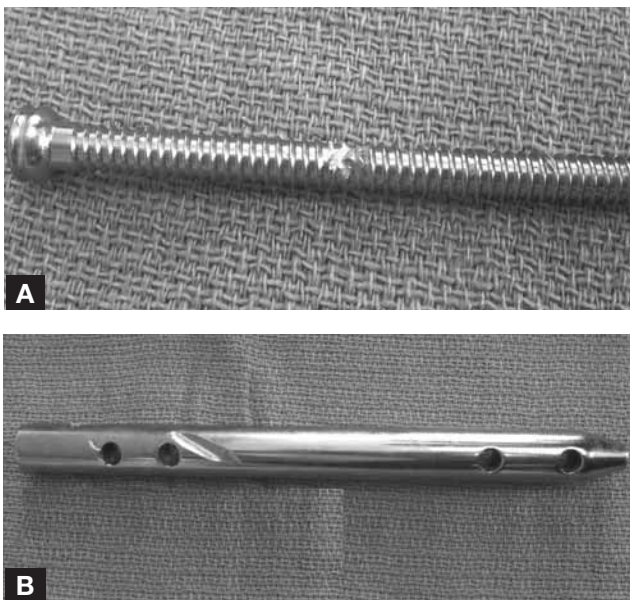
Figure 5. Damage to (A) distal transverse locking screw and (B) nail adjacent to more proximal distal transverse locking screw hole.
