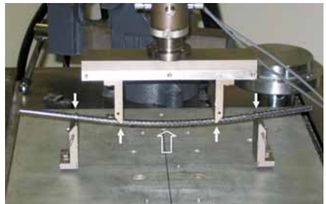
Figure 2. Loading points (solid arrows) and loading zone (open arrow) of loading jig.
