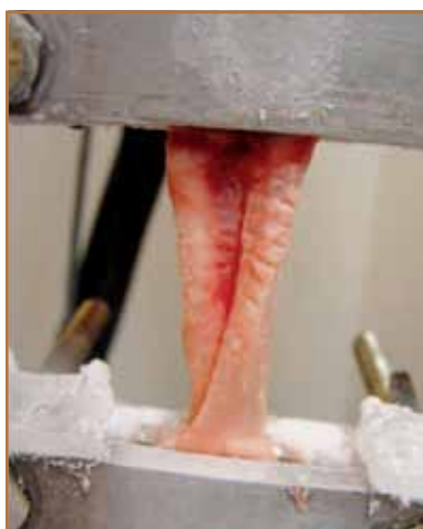
Figure 3. Graft positioned for testing in cryoclamps proximally and distally. Unsupported gauge length (35 mm) used for each sample. Indentations from placement of interference screw are visible on graft.
