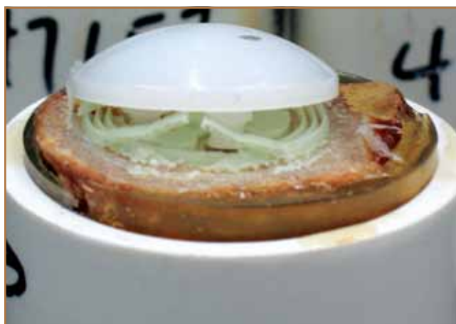
Figure 2. Patella with patellar component after shear testing.
