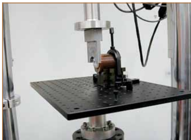
Figure 1. Materials testing machine (MTS; MTS Systems Corp, Eden Prairie, Minnesota) with guillotine-type shear-testing apparatus and patella mounted in polyvinyl chloride pipe.
