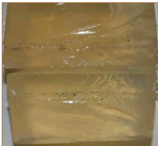
Figure 4. Gel shot with .22 caliber bullet cut in half along projectile pathway demonstrating gross contamination with denim.
