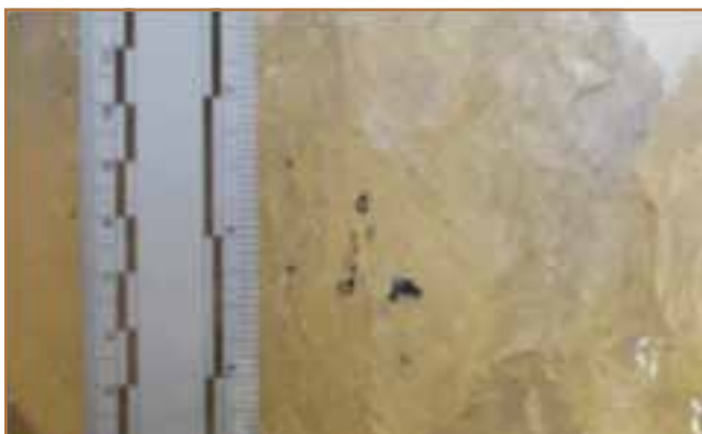
Figure 7. Gel shot with a .45 caliber bullet with denim contamination.
