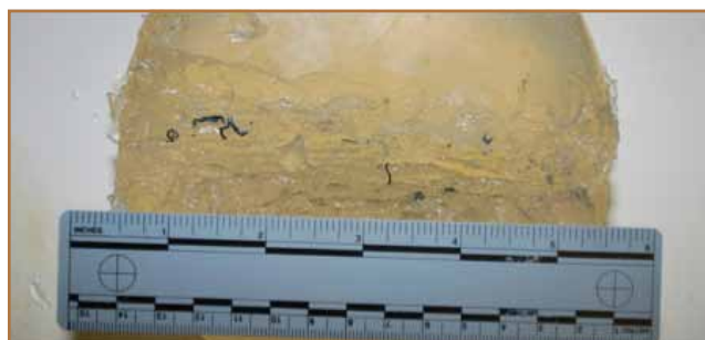
Figure 5. Overview of a gel shot with .38 caliber bullet demonstrating gross contamination with denim throughout entire pathway as well as entrance and exit wound.
