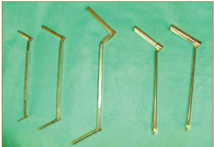
Figure 1. Various sizes of commonly available drill sleeves and tap sleeves.
