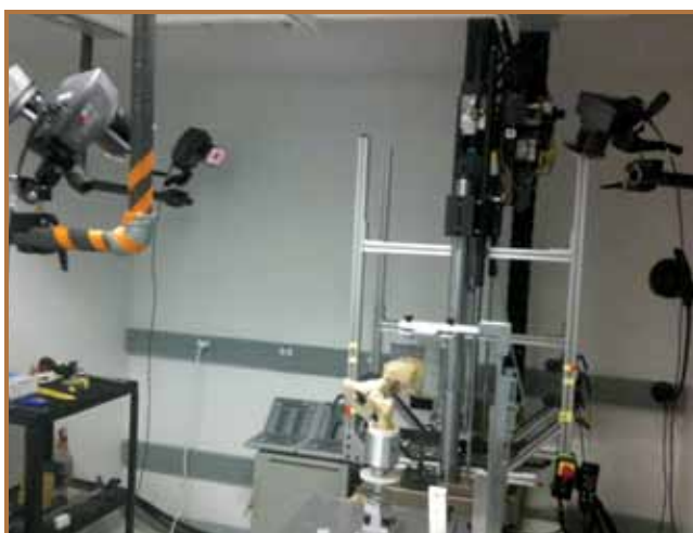
Figure 1. Motion tracking system with loading apparatus mounted on x-y displacement table.
