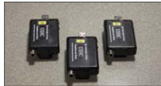
The pager-size badges that are worn by health care workers wirelessly detect the use of tagged hand-hygiene dispensers for alcohol-based sanitizer or soap. The devices automatically log the date, time, and length of use.
