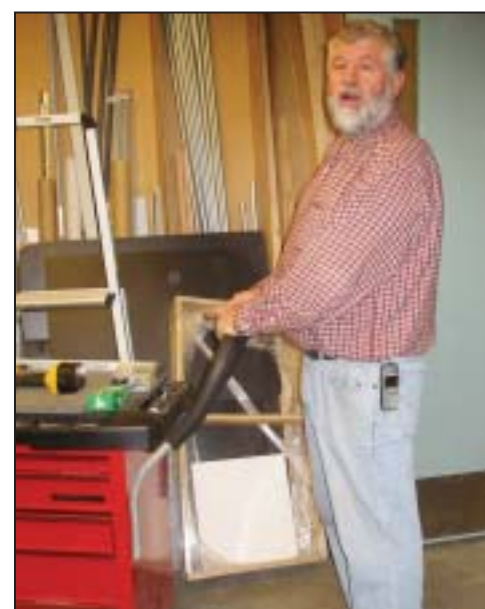
With a raised handle on the cart, the user can stand upright and move it more easily.
