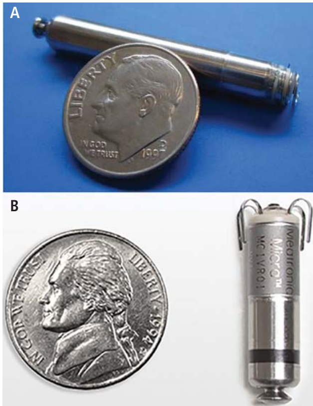
FIGURE 2. Leadless pacemakers (A) Nanostim and (B) Micra.
