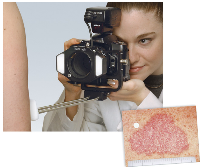
Figure 10 A close-up accessory assures consistent camera position and includes a measurement scale.
