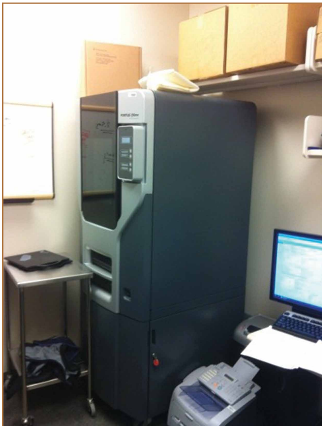
Figure 8. Our in-office 3-dimensional printer sits in corner adjacent to clinical workstation. Relatively little office space is required for machine’s 33×29-in footprint.
