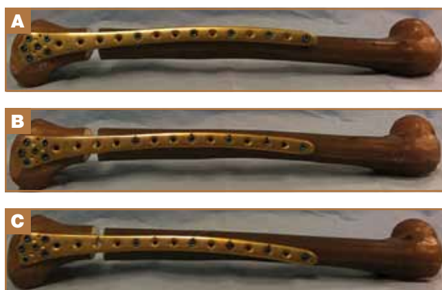
Figure 1. Fourth-generation femoral synthetic composite bones (Sawbones; Pacific Research Laboratories, Vashon, Washington) with 13-hole Less-Invasive Stabilization System (Synthes, Paoli, Pennsylvania) plate in (A) correct position, (B) anterior position, and (C) posterior position.
