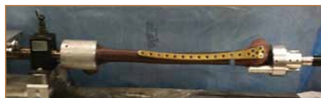
Figure 3. Setup for torsional simulated loading.
