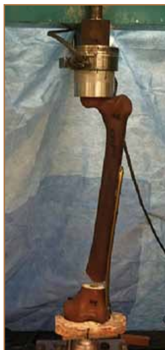
Figure 2. Setup for axial simulated loading.
