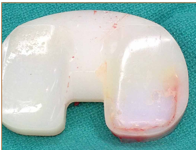
Figure 5. The modular tibial liner shows severe wear including pitting, cracking, and delamination.
