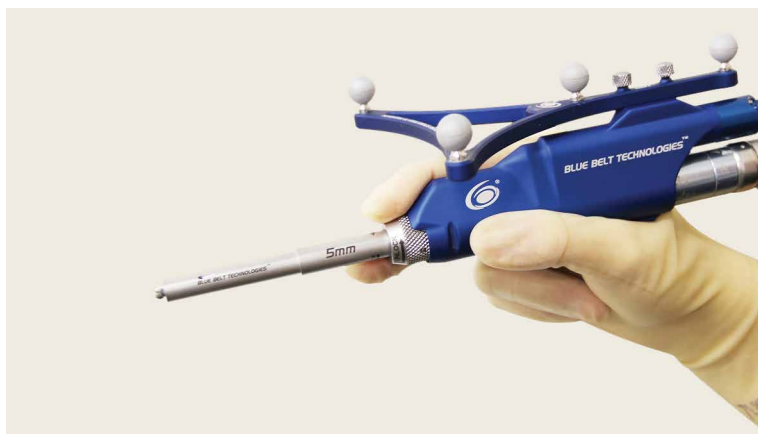
Figure 4. The robotic-assisted Navio Precision Free-Hand Sculptor (PFS) system (Blue Belt Technologies).
