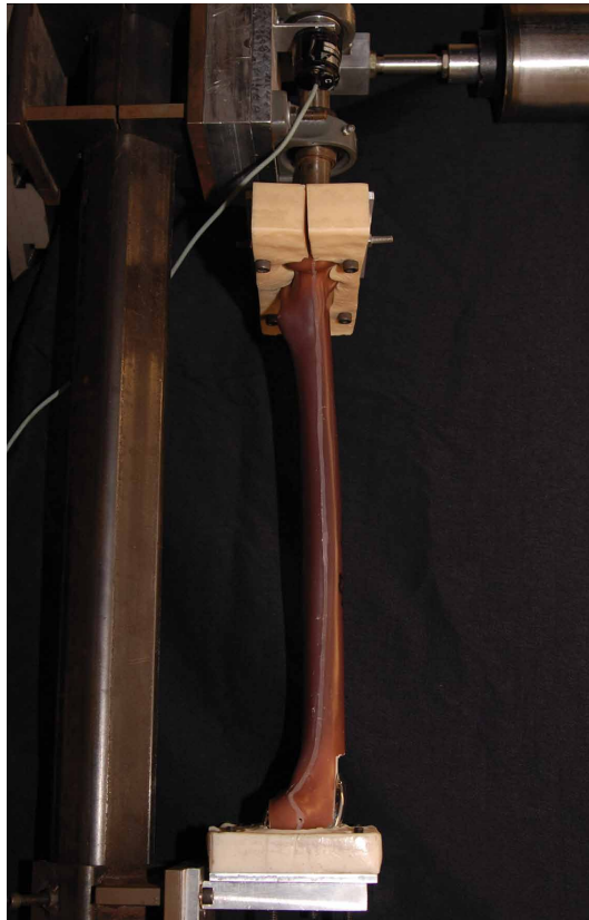
Figure 1. Test specimen loaded on torsional testing apparatus.
