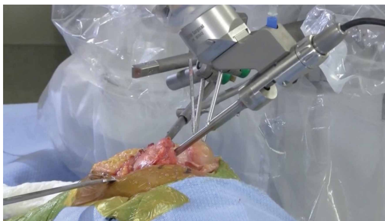
Figure 2. The TCAT system actively milling the femoral canal during a total hip arthroplasty procedure.
