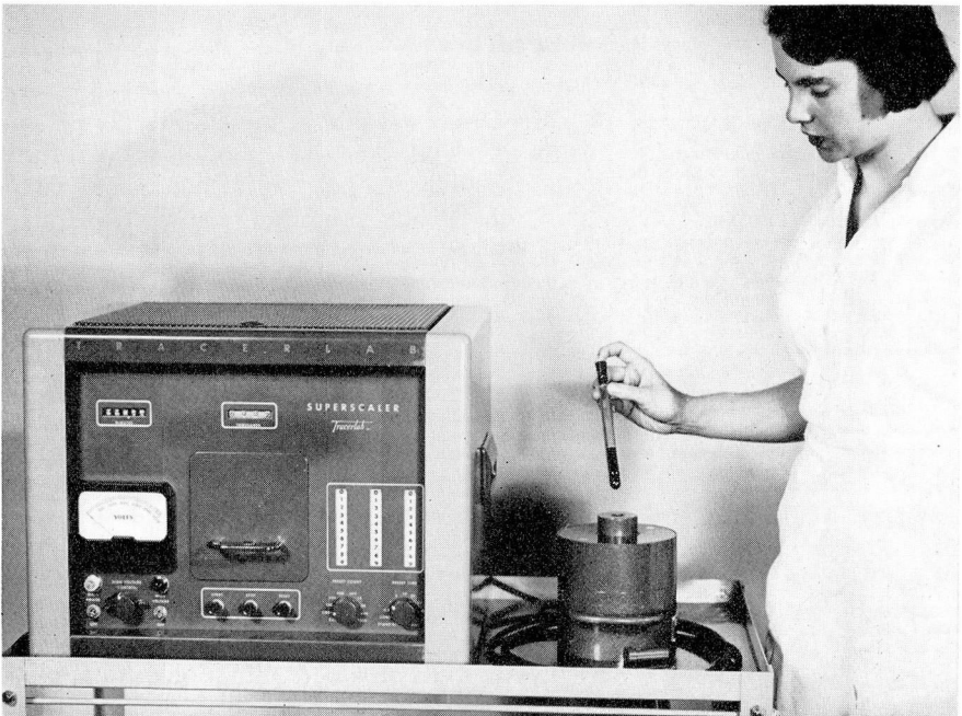
Fig. 1. Test tube being placed in the well counter where its radioactivity will be measured on the scaler.
