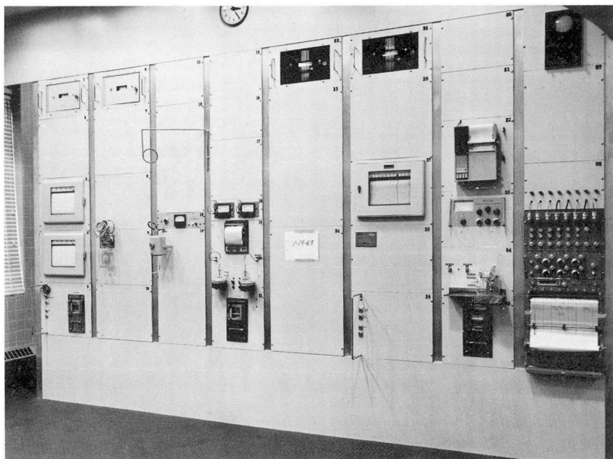
Fig. 16. Analytical wall designed for continuous direct monitoring of patients. (Courtesy of Leland C. Clark, Jr., Ph.D., Medical College of Alabama, Birmingham, Alabama.)
