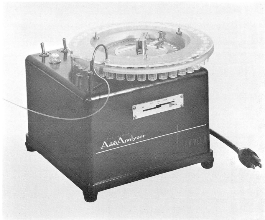
Fig. 5. Sample module. Tests-per-hour lever regulates the rate at which sample crook lifts and table turns. (Courtesy of Technicon Instruments Corporation, Chauncey, New York.)
