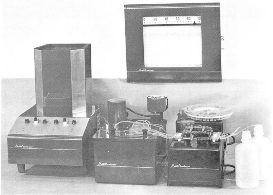
Fig. 12. Flame photometer. Recorder is equipped to record simultaneously sodium and potassium levels. (Courtesy of Technicon Instruments Corporation, Chauncey, New York.)
