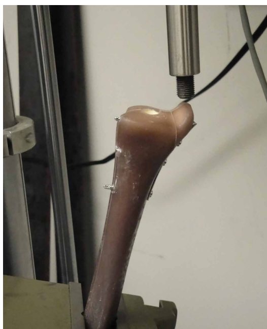
Figure 2. Offset-axial loading at 17° from vertical.
