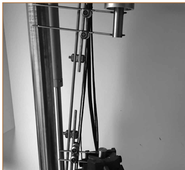
Figure 5. Construct in MTS testing apparatus (MTS 858 Mini-Bionix Test System).
