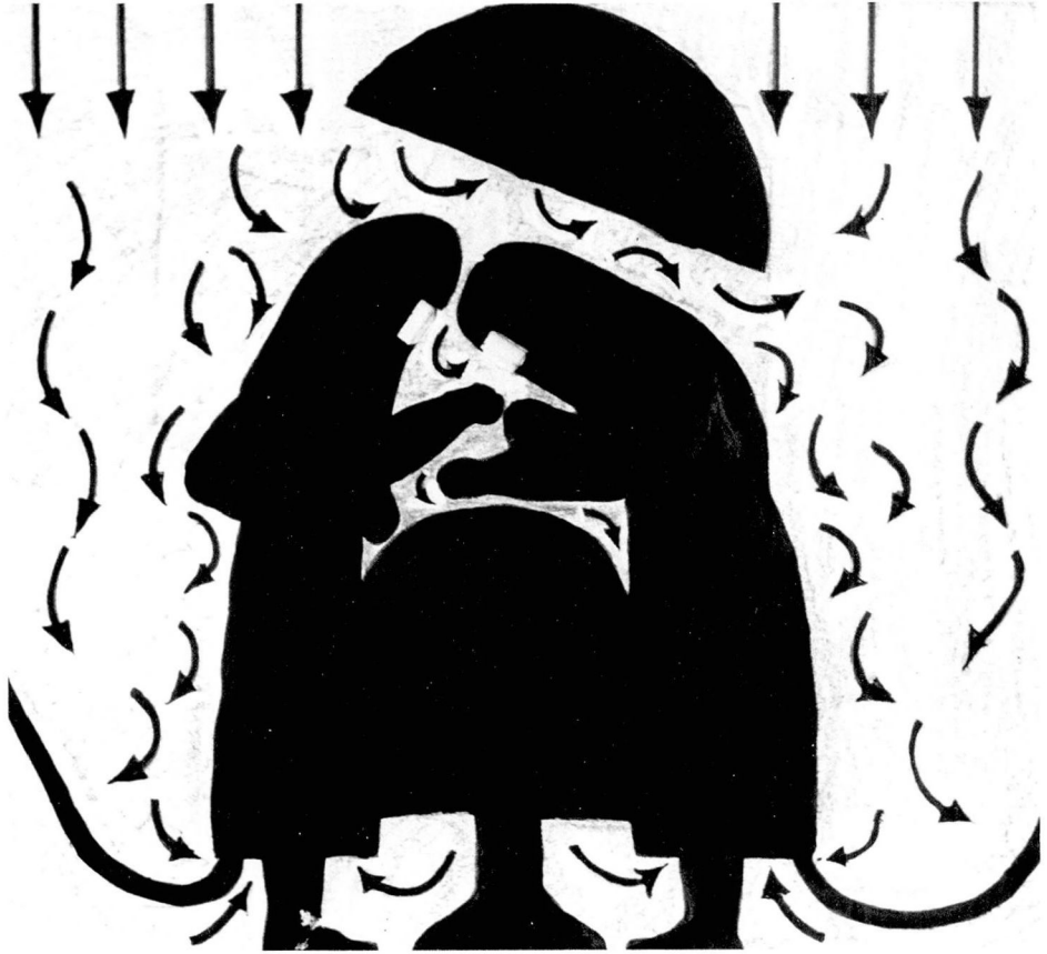
Fig. 7. Semiturbulent air flow combined with body exhaust system. Turbulence not sufficient to permit currents rising from the floor. Perfect overhead surgical lighting possible.
