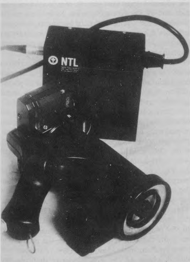
Figure 1. The cerviscope, or special 35-mm camera and power unit designed for cervicography.
