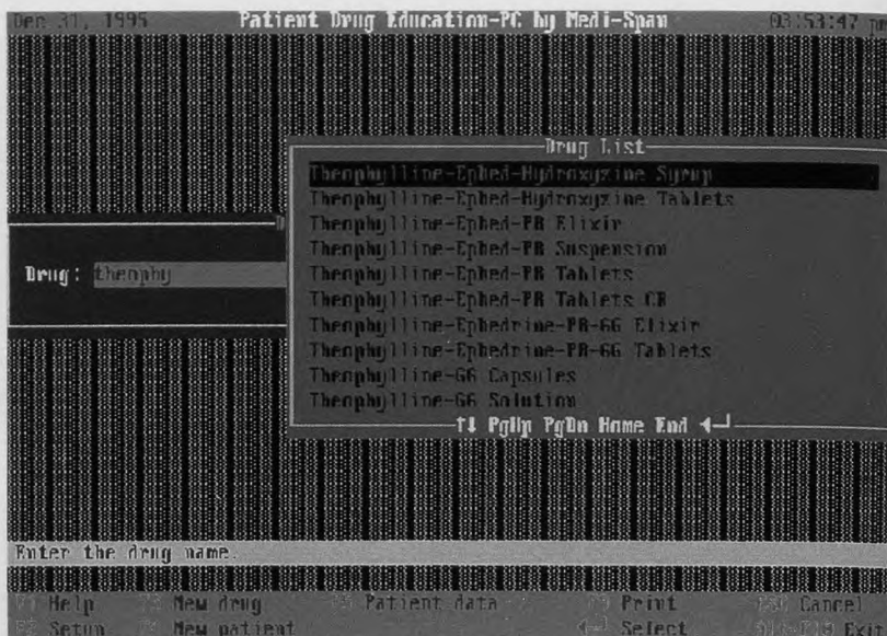
Figure 1. User types drug name, then presses Enter key. Alphabetized drug list pops open to appropriate point, from which user can use page and cursor keys to scroll to the desired selection.
